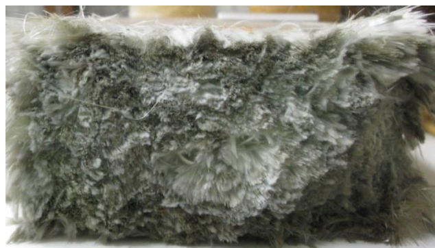
Figure 1. 50 percent by volume ratio of glass fibres in the cross section of the FFU- railway sleeper.
