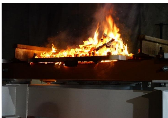
Figure 7. Fire test on open steel beam construction (here: Fire on the upper surface of the bridge track).
