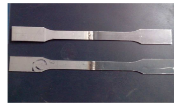
Figure 4. Tensile Test Specimens.
