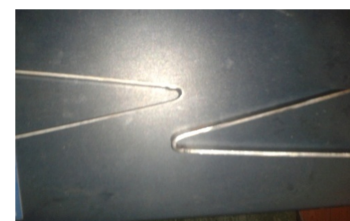
Figure 7. Test Specimens showing satisfactory weld properties.
