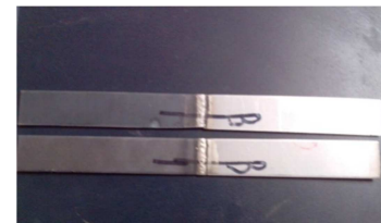
Figure 5. Test specimens for bend tests.
