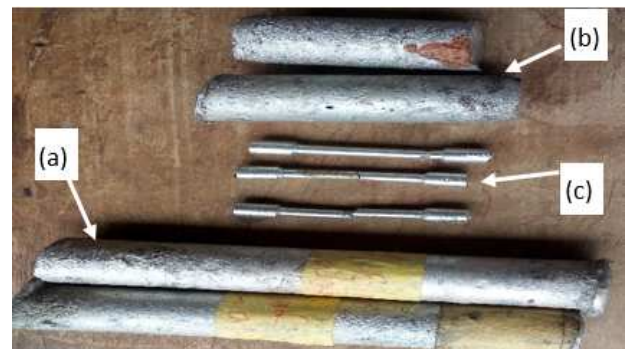
Figure 4. Samples of (a) quenched aluminium alloy rods (b) cut aluminium alloy rods and (c) machined specimens.
