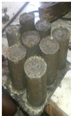
Figure 2. Briquettes (dried at temperature 28°C) after ten days.
