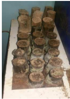
Figure 1. Briquettes (wet) immediately after extrusion from machine.
